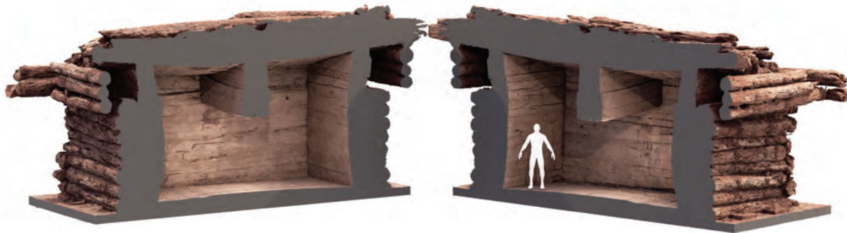
Figure 38: Cut-away view of the Tumulus MM tomb chamber. Digital model by Matthew Harpster’s team and Emin Erdal.
